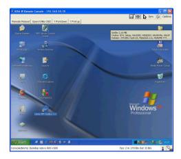
The upper part of the Remote Console window contains a control bar. The remote command buttons on the left side can be configured except for the Remote Reboot (CTRL-ALT-DELETE). When viewing the icons on the right side you will see the current state of the Remote Console and be able to adjust the local Remote Console settings. There are several options to choose from, below is an introduction to the most important ones. Please refer to the User Manual for further options and information.
