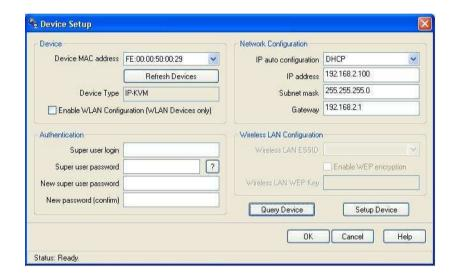
On the upper left corner, the MAC address of the KVM IP ACCESS MODULE is displayed. To detect the MAC address, press the **Refresh Devices** button. The displayed MAC address should correspond to the printed address shown on the label on the base of the IP module.
